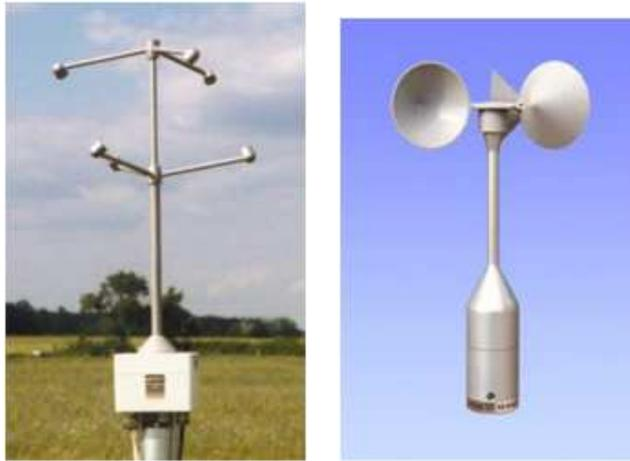
Figure 15. Left: The Metek Sonic. Right: The cup anemometer.
